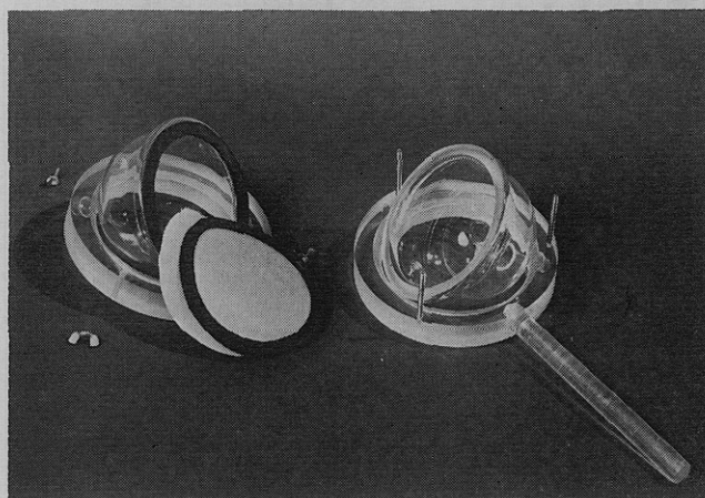
Figure 1B. Disassembled filtration apparatus showing Miracloth filter, gaskets, and polystyrene frame
